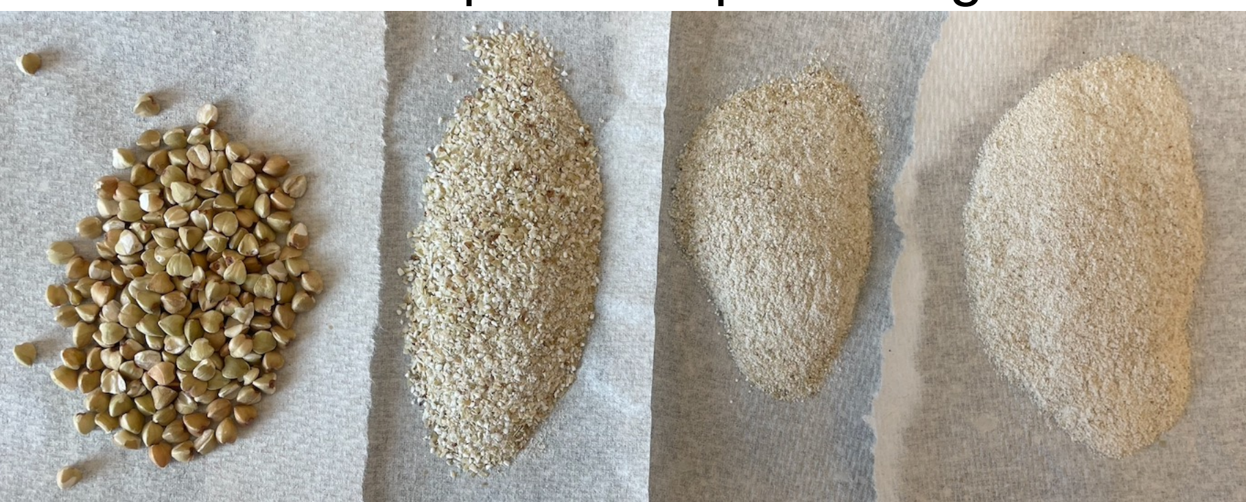
Grind sizes tested. From left to right: whole groats, #20 sieve, #40 sieve, #60 sieve.
